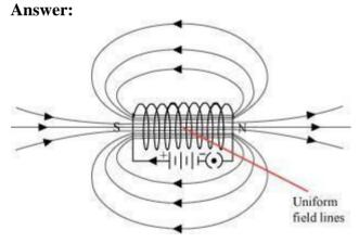
The magnetic field lines inside a current-carrying long straight solenoid are uniform.
