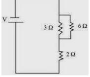
Here, 6  $\Omega$  and 3  $\Omega$  resistors are connected in parallel. Therefore, their equivalent resistance will be given by
