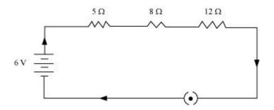
2. Redraw the circuit of question 1, putting in an ammeter to measure the current through the resistors and a voltmeter to measure potential difference across the 12  $\Omega$  resistor. What would be the readings in the ammeter and the voltmeter?
