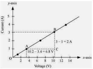
The slope of the line gives the value of resistance (*R*) as, Slope = 1/R = BC/AC = 2/6.8*R*= 6.8/2 =  $3.4 \Omega$ Therefore, the resistance of the resistor is  $3.4 \Omega$ .
