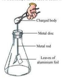
It consists of a metal rod. At one end of the rod, two leaves of aluminium foil are fixed and at the other end, there is a metal disc. The leaves of aluminium foil are placed inside a conical flask and the flask is corked to isolate the leaves from air.
