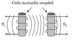
Let  $n_1$  be the no. of turns per unit length of  $S_1$ ,  $n_2$  be the number of turns per unit length of  $S_2$ .
