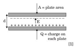
A parallel plate capacitor consists of two large plane parallel conducting plates separated by a small distance d. The two plates have charges q and -q and distance between them is d.
