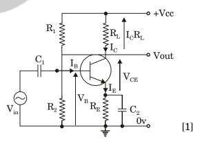
**Working:** If a small sinusoidal voltage is applied to the input of a CE configuration, the base current and collector current will also have sinusoidal variations. Because the collector current drives the load, a large sinusoidal voltage  $v_0$  will be observed at the output. [1]
